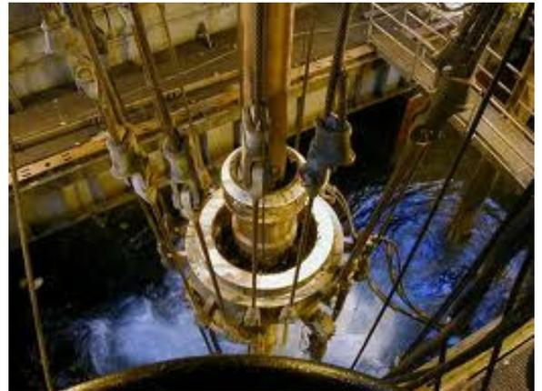
The wedge socket is an application for special load pins. The pins are designed for the application and for the moon pool area it has to be marine resistant.
